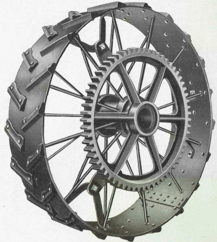
Drive Wheel with Lug-Gear Attached
